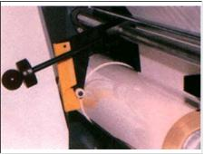
Precision pre-slitting of laminate to exact widths with slitting attachment - Standard Equipment.
