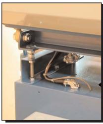
Elevated Base Lowers table away from screen for printing on plywood, glass, styrofoam, plastic extrusions or other thick substrates
